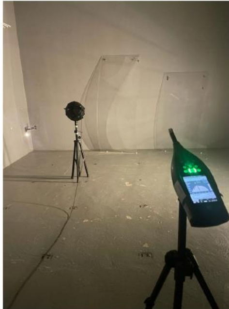
Figure 1: Reverberant chamber assembly with source only
