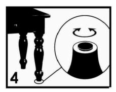
Some furniture comes with height adjusment knobs underneath each leg. To lower or to raise each leg, you need to turn clockwise or counterclockwise, respectively.
