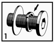
When lock or spring washer is used in an assembly, please make sure the lock or spring washer is placed between the larger flat washer and the head of the screw or bolt.
