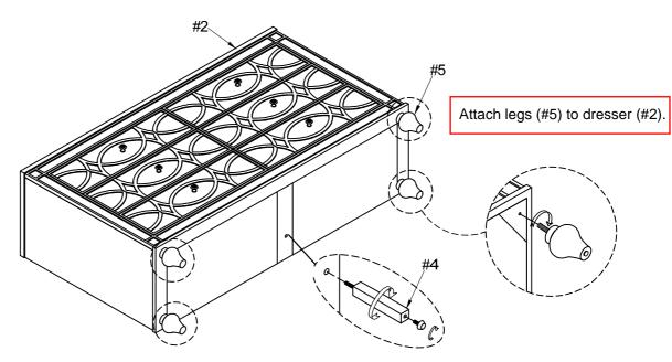
Attach support legs (#4) to dresser (#2), then adjiust leveler of support leg (#4) according to ground level.
